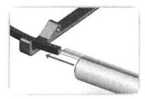
While holding the thread on the shaft with the thumb and the forefinger, start to make it slide in the frame.
