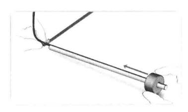
Then, by holding the frame, push the cylinder to make the thread slide in the frame.
