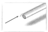
Introduce the needed length of thread in the shaft. As shown on the picture, the size is not often symmetrical, place the smallest diameter in the groove.
